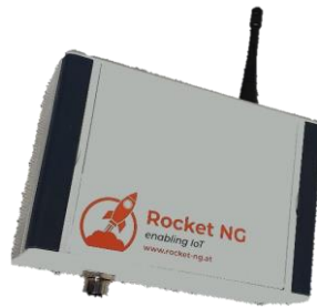
Figure 2: Autonomous sensor node with external antenna.
